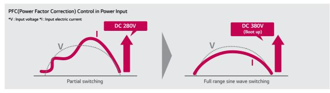
The operating voltage is increased from DC 280V to DC 380 V.
