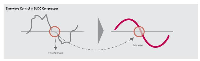
With sinusoidal wave function of the voltage, the sine wave makes the function more soft and efficient.
